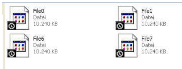
[Fig. 1.6 – Migrated files marked with offline bit on Windows XP node]
